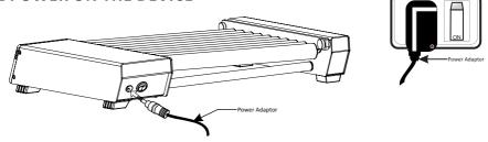
After connecting the power adaptor to back side of device, switch the main power supply to "ON" & then switch ON the device from rear side end. Make sure that tubes are loaded properly before use. Do not start the device if the hinge is open.
