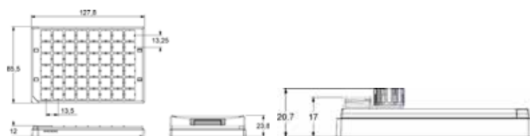
Micronic 48-1 rack dimensions and tube in rack dimensions 1.00ml externally threaded tubes with Screw Caps.
